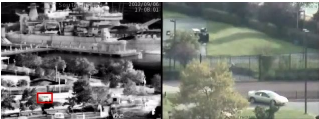
Long-range smart thermal cameras detect (left) and auto-zoom PTZs for assessment (right)
